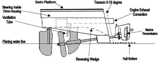
Our innovative drive housing does many things, it supports the rudder, shaft tube and exhaust system, it also provides on the under side a unique wedge that directs the reversing water flow down and under the hull thus giving excellent reverse thrust and control.
